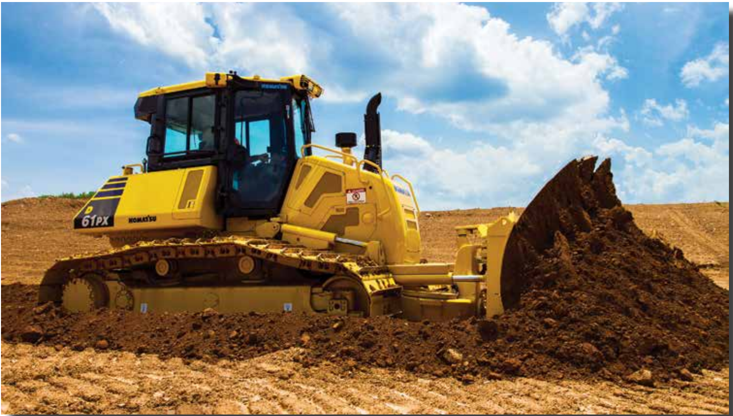
Gideon Excavating uses the Komatsu D61EX dozers for building pads and other site-work projects.
